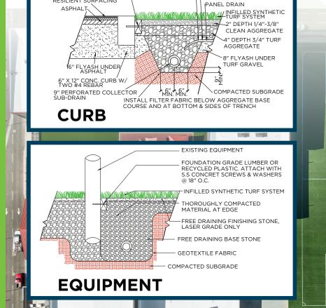
PRESSURE TREATED 2X4 ANCHOR TO CONCRETE CURB W/ 1/2"Ø STAINLESS STEEL EXPANSION ANCHORS
